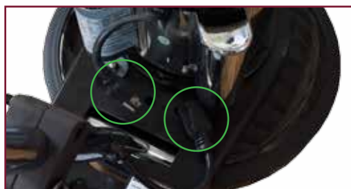
Convenient Unplug to disconnect motor for service
