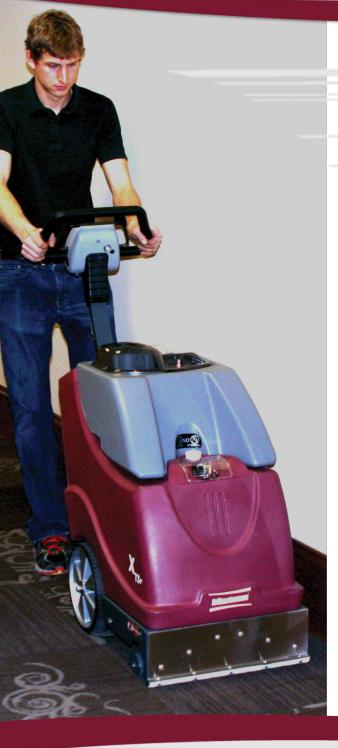
The X17 Series combines powered brush agitation with high pressure spray and a wide 17" vacuum shoe for unparalleled maintenance cleaning of carpets in offices, schools, hotels, medical centers, retail centers and more.
