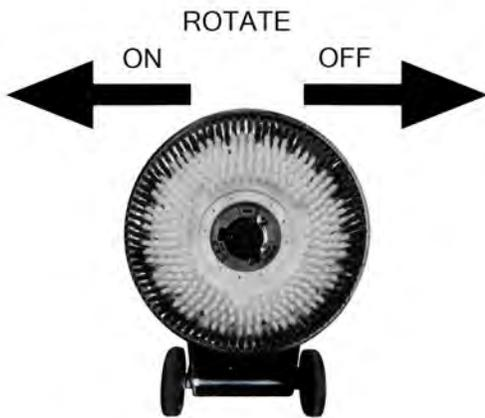
**WARNING: Never change a brush or pad driver, while the machine is connected to a power source. Always, unplug machine.**
