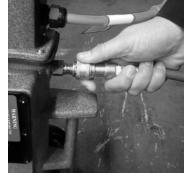
5. Connect the power cord on the heater to the female twistlock plug located on the rear of the R100H.
