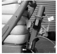
3. Connect your heater's inlet hose (#1 on page 7) to the machine's outlet quick disconnect (#6 on page 6).
