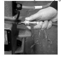
5. Your R500H has two cords- One for the Extractor and one for the heater. Each cord requires a separate 15AMP circuit. Connect your 50FT power cord to the twist lock pigtail on the heater (#4 on page 7). Plug another 50ft power cord to the twist lock pigtail on the back of the machine (#6 on page 6)
