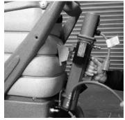
3. Connect your heater's inlet hose (#1 on page 7) to the machine's outlet quick disconnect (#7 on page 6).
