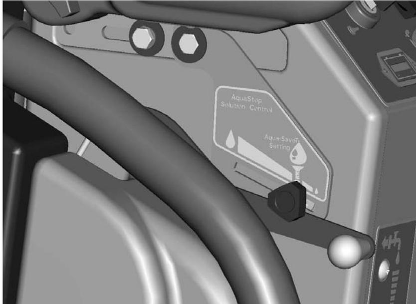
In order to consistently conserve water when using Aquastop brushes, the guide will stop the solution control lever at a low rate setting. This setting may be adjusted by loosening the knob, adjusting the lever, and retightening the knob. Slide the knob all the way forward to dispense maximum solution.
