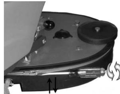
3. The splash guard may be moved up or down as the brush/pad wears by loosening the clamp on the back side of the deck with a flathead screwdriver or 9/32" (7mm) socket, then slide the splash guard to the desired height & retighten the clamp.
