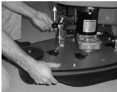
1. Brush Deck may be tilted up for easier brush installation/removal & to clear steep ramps. Lift the handle on the upper lever which connects the brush deck to the machine, tilt the deck up, release the handle & the lever will lock into place. Lift the handle again to move the deck back to horizontal.
