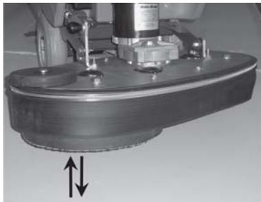
2. Brushes are installed/removed by hand. Push each brush up onto the hub until it "clicks". To remove, pull down on the edge of each brush.
