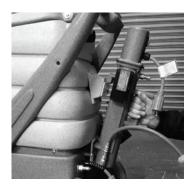
3. Connect your heater's inlet hose (#1 on page 11) to the machine's outlet quick disconnect (#6 on page 10).
