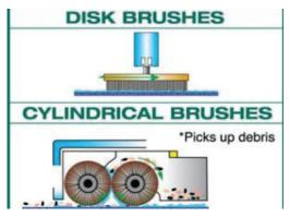
Cylindrical scrubbing utilizes counter rotational brushes that mechanically lift debris while cleaning. Brushes turn in opposite direction of each other and facilitate pre sweeping for many applications. It is especially effective for all types of three dimensional flooring with it's unique ability to clean deeper in uneven surfaces.
