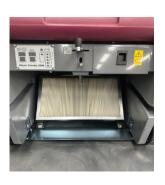
Polyester pleated panel filter that allows dustless sweeping operation. No tools required service and removal.
