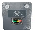
After adjusting the brush height, the machine will detect within seconds when you can start cleaning — "when it's green, it's time to clean".
