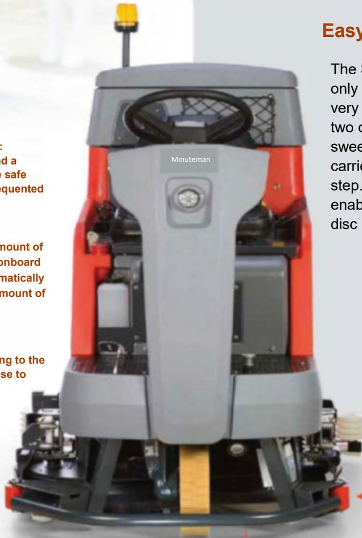
Robust bumpers both at the front and rear provide effective collision protection and increased safety.
