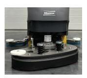
The E26 ECO is equipped with a water diversion valve which enables our proprietary "Aqua Saver" green technology to optimize the consumption of water and chemical. Partnering aqua stop brushes with aqua saver solution control creates 19 gallon productivity in a 12 gallon platform. The result is less filling and emptying of the tank and more efficient cleaning with a greater ROI.
