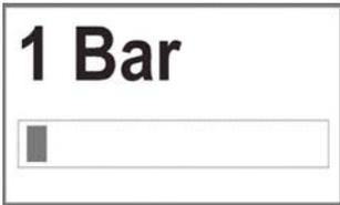
The battery needs charging, there is a bad connection to the battery or dependent on programming, may indicate that the battery lockout function is active and the controller is in a restricted mode of operation. Check the connections to the battery. If the connections are good, try charging the battery.
