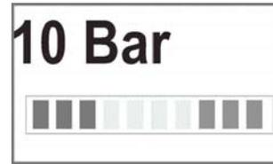
An excessive voltage has been applied to the controller. This is usually caused by a poor battery connection. Check the battery connections.
