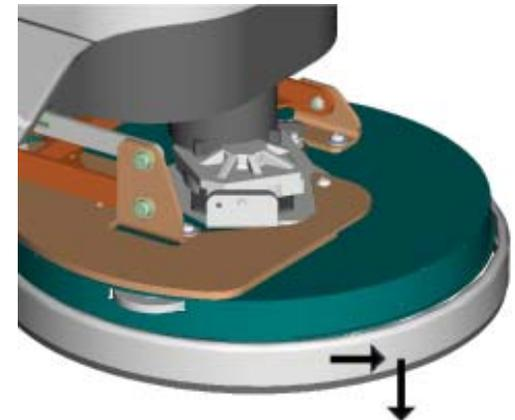
With brush removed & deck raised, Remove skirt for cleaning by pulling forward, then down over the edge of the deck.
