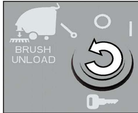
2. Momentarily turn the key (1 to 2 seconds) to the "Brush Unload" position then let the key return to the off (O) position.
