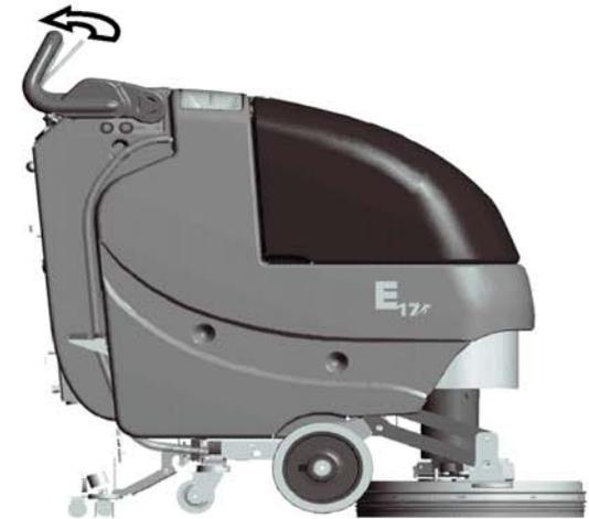
3. With the key turned on, pull the bail handle to engage the scrub brush onto the scrub deck.
